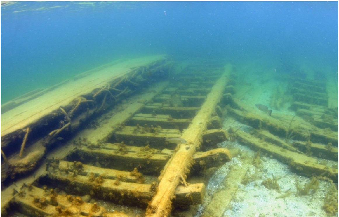
Figure 18. The bilge of *Grape Shot* and the fallen centerboard trunk
