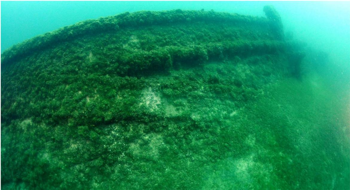
Figure 7. *S.C. Baldwin*'s wooden hogging arch, comprised of three individual timbers
